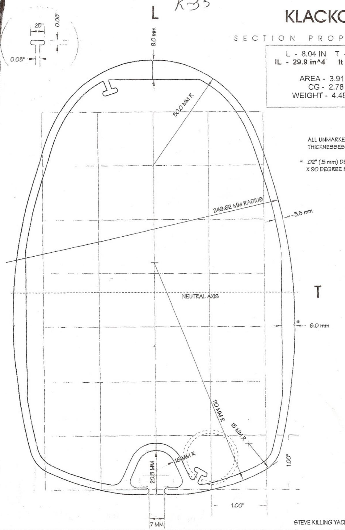
ALL UNMARKED WALL THICKNESSES ARE 3.5 MM
