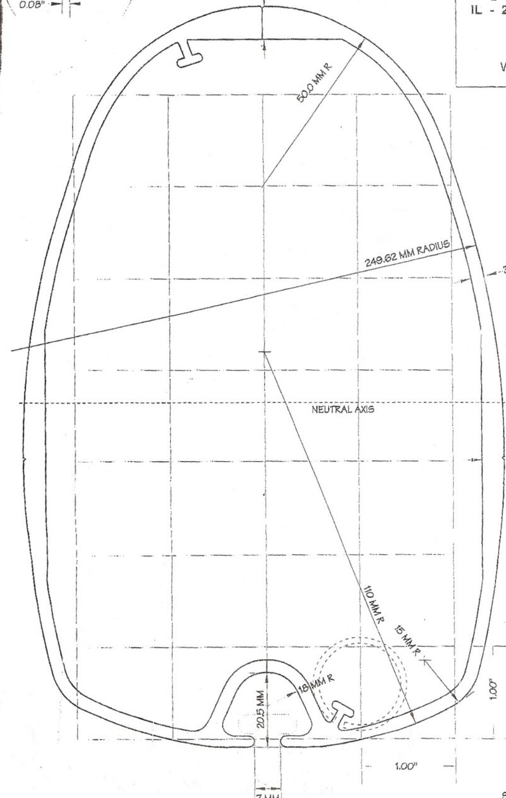
ALL UNMARKED WALL THICKNESSES ARE 3.5 MM
